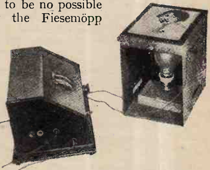
Fig. 2.—“Simple experimental arrangement of the Fiesemöpp Televisor.”
