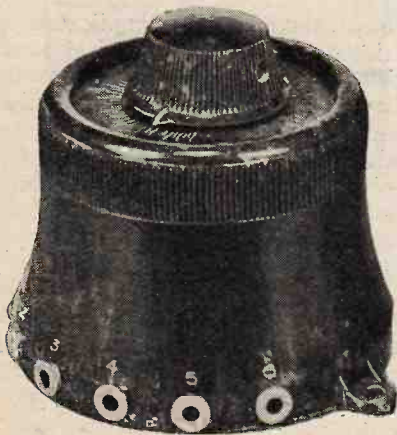
By interconnecting the sockets, the Brownie wave-trap can be converted into a selectivity unit.
